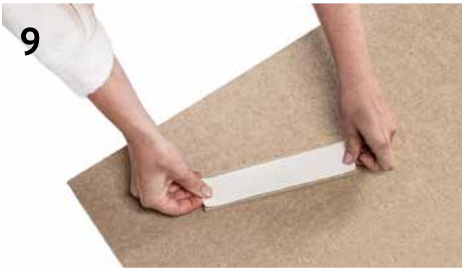
9 Position the double sided tape to the back of the felt spacer
