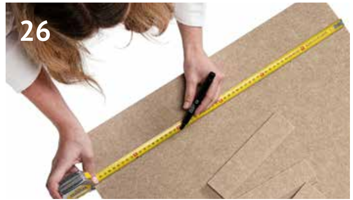
26 Check if the distance between the marked points is 20 centimeter (size of the felt spacer)
